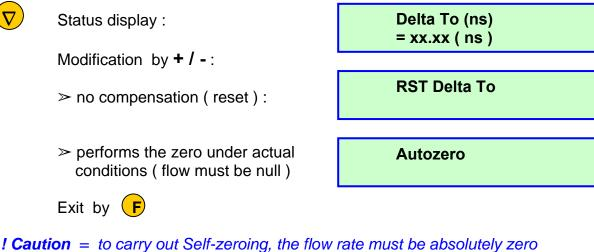
! Caution = to carry out Self-zeroing, the flow rate must be absolutely zero while the display indicates « \* dTo \* ».
